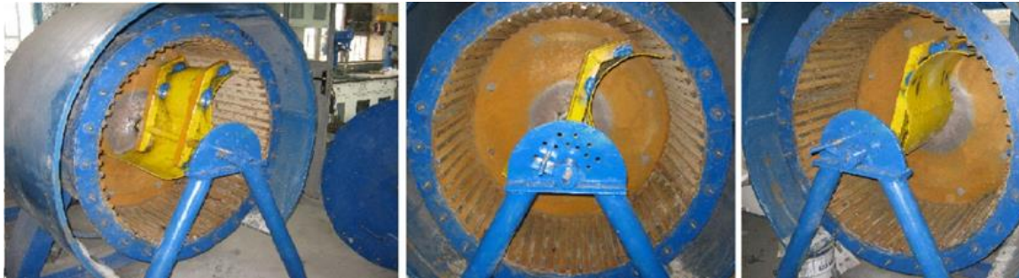
Fig. 3. Lateral device that installed in pilot SAG mill to prevent cascading motion.
