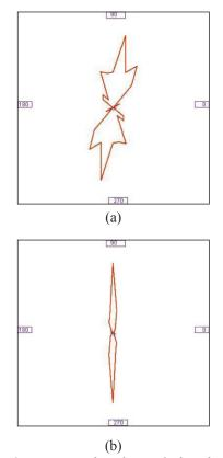
Fig. 10. Orientation of voids just before fracture, in which degree of  $90^{\circ}$  is tensile direction,(a) DP780 and (b) DP980 steel.
