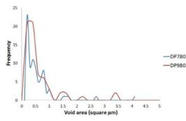
*Fig. 9. Frequency of void surface Area distribution in DP780 and DP980 steels, behind the fracture surface.*
