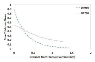
*Fig. 7. Strain gradient in longitudinal direction in DP980 and DP780 steels.*
