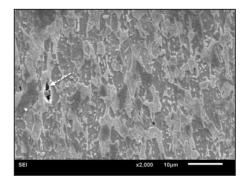
Fig. 4. Formation of voids at inclusions in DP980 steel, indicated by arrow.
