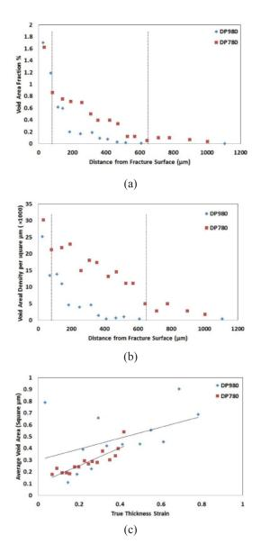
Fig.8. Variation of (a) void area fraction, (b) void areal density and (c) void average area versus distance from fracture surface for DP780 and DP980 steel.
