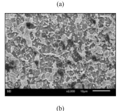
Fig. 2. Microstructure of (a) DP780 and (b) DP980 steel.
