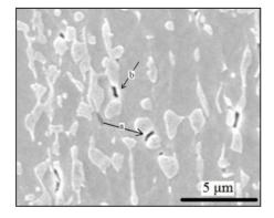
Fig. 3. Void nucleation by martensite cracking (showed by arrow "a") and between martensite particles located at the ferrite grain boundaries, by interface decohesion (showed by arrow "b"). This figure is related to DP780 steel; however, the same behavior was observed in DP980 steel.
