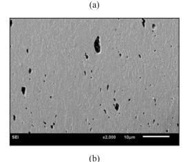
*Fig. 6. Accelerated void nucleation just before fracture surface for (a) DP780 and (b) DP980 steel.*
