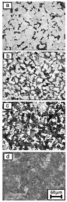
Fig. 2. Metallographic images of AISI a) 1015, b) 1035, c) 1045, d) 1080 steel after full annealing.
