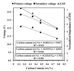
*Fig 5. The relation between carbon content of steels and eddy current outputs at 650 Hz.*
