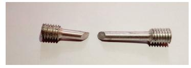
Fig. 6. A sample after tensile test.
