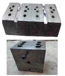
Fig. 4. Schematic illustration of inner part of the mold.
