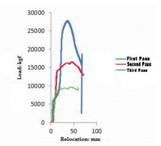
Fig. 7. Extruded Al6061 in the first, second and third passes.
