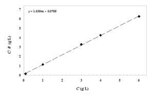
Fig. 6. Langmuir adsorption isotherm for API 5L carbon steel in the absence and presence of the Nettle extract in 0.5  $M H_2SO_4$
