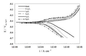
Fig. 3. Tafel polarization curves of API 5L carbon steel in 0.5  $M H_2SO_4$  in the absence and presence of different concentrations of the Nettle extract.
