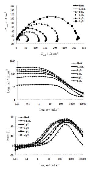
Fig. 4. EIS plots of API 5L carbon steel in  $0.5 M H_2 SO_4$ in the absence and presence of different concentrations of the Nettle extract exemplified as: (a) Nyquist, (b) bode modulus, and (c) bode phase angle plots.
