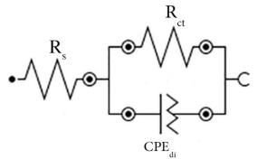
Fig. 5. The best equivalent circuit used to model the experimental EIS data of API 5L carbon steel in 0.5  $M H_2 SO_4$  in the absence and presence of different concentrations of Nettle.
