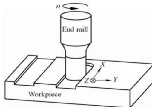
Fig. 3. Detailed milling coordinate system. X, Y, and Z direction correspond to feed, perpendicular and axial, respectively.
