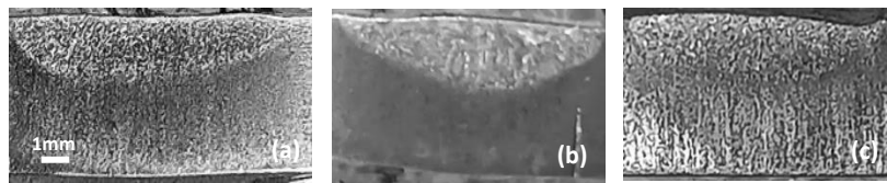
Fig. 1. Macrograph of welding samples (a) TIG (with Ar gas) (b) A-TIG CeO 2 (c) A-TIG CeO 2 +5% N 2 .
