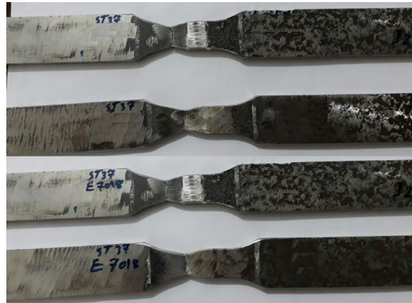
Fig. 7. The fracture zone of the two tensile samples.
