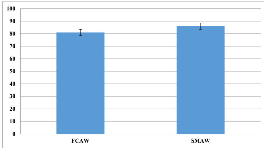
Fig. 9. Bar graph of the average energy of FSAW and SMAW.
