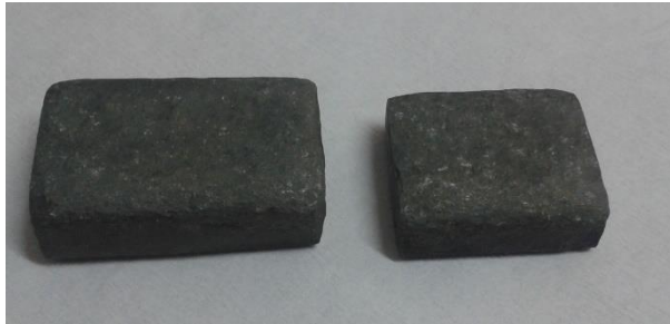
Fig. 3. Two specimens were made from ductile steel to measure wear.
