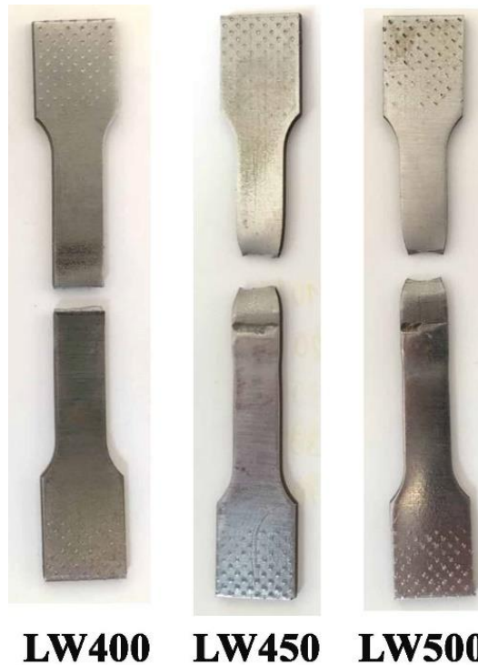
Fig. 9. Failed samples of the welded joints.
