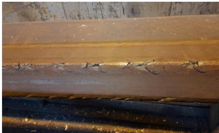
Fig. 1. Edge cracks created during hot rolling of AISI304L steel.
