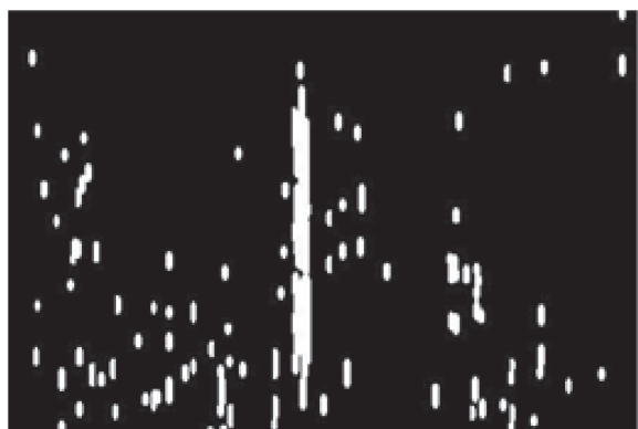
Fig. 12. Linking the gaps along the crack.
