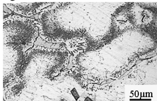
Fig. 9. Precipitation in Inconel 657 HAZ.
