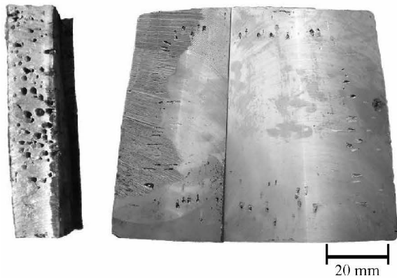
Fig. 3. Cross Section of Casting Ingot and Transverse View of Porous Region.
