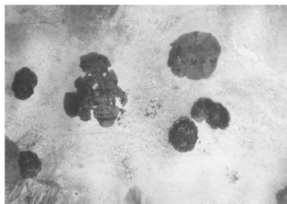
Fig 11. Microscopic image of pearlitic samples cooled in air after 200 cycles. Near spherical cementite can be seen in the image.
