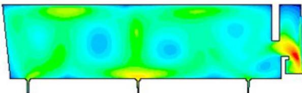
Fig. 6. Field of liquid steel flow in the tundish with turbo stop and a weir with 300 mm distance from center of tundish.
