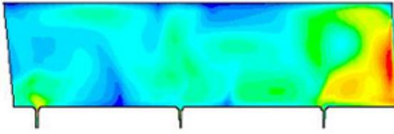
Fig. 2. Field of liquid steel flow in the tundish without any control device.
