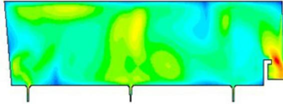
Fig. 3. Field of liquid steel flow in the tundish with turbo stop.
