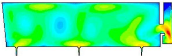
Fig. 5. Field of liquid steel flow in the tundish with turbo stop and a weir with 200 mm distance from center of tundish.
