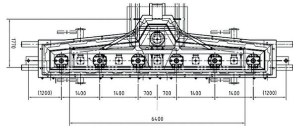
Fig. 1. Geometry of six-strand tundish considered in the present study.
