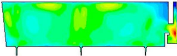
Fig. 4. Field of liquid steel flow in the tundish with turbo stop and a weir with 100 mm distance from center of tundish.
