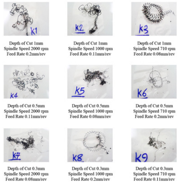
Fig. 9. Chip morphology obtained in facing operation of 55Cr3 steel bars.
