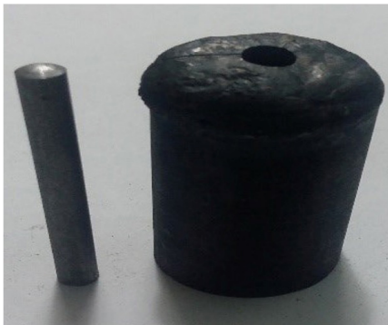
Fig. 4. Pin used in pin on the disk test Manufactured from the welded zone.
