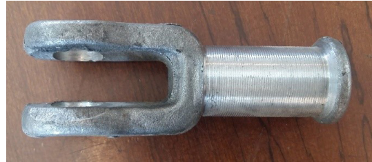
Fig. 5. Typical product produced with the hot forging process.
