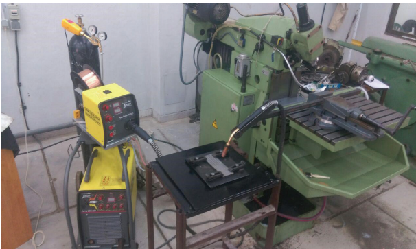
Fig. 2 Gas metal arc welding set-up.
