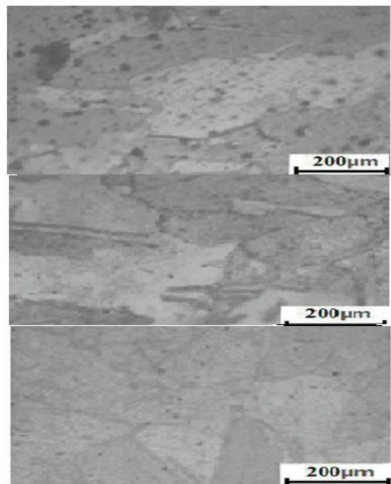
Fig. 9. Pictures of grain size samples annealed first pass and second pass metallography, respectively from left to right.
