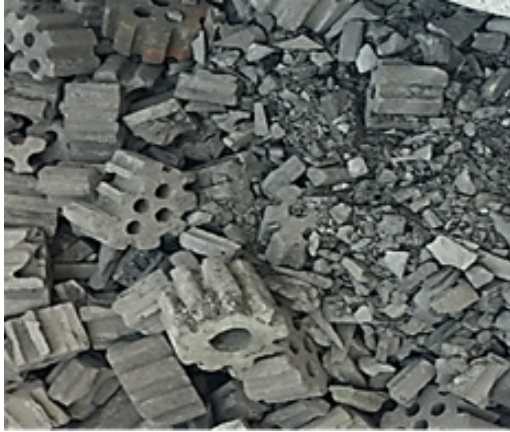
Fig. 2. Crushed catalysts discharged from the destroyed tube.
