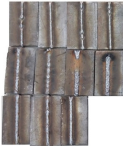
Fig. 3. NE-GMAWed Experimental samples.
