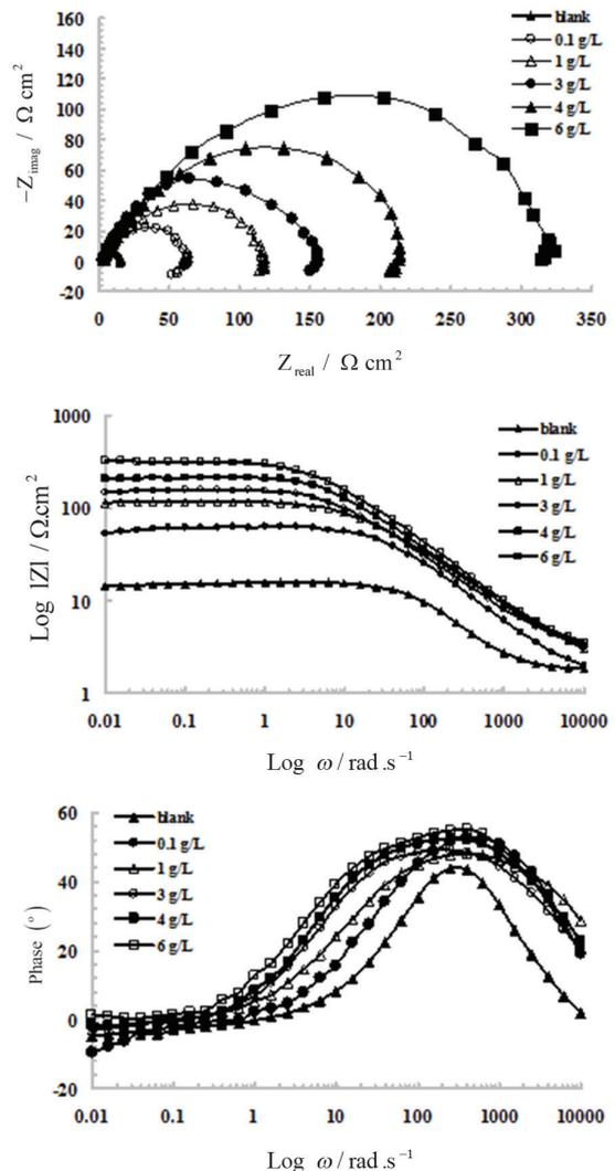
Fig. 4. EIS plots of API 5L carbon steel in 0.5 M H<sub>2</sub>SO<sub>4</sub> in the absence and presence of different concentrations of the Nettle extract exemplified as: (a) Nyquist, (b) bode modulus, and (c) bode phase angle plots.
