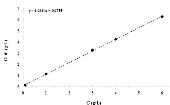
Fig. 6. Langmuir adsorption isotherm for API 5L carbon steel in the absence and presence of the Nettle extract in 0.5 M H<sub>2</sub>SO<sub>4</sub>.
