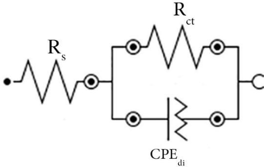
Fig. 5. The best equivalent circuit used to model the experimental EIS data of API 5L carbon steel in 0.5 M  $H_2SO_4$  in the absence and presence of different concentrations of Nettle.
