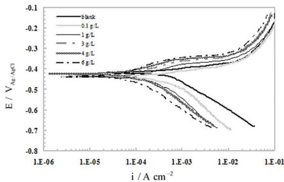
Fig. 3. Tafel polarization curves of API 5L carbon steel in 0.5 M H<sub>2</sub>SO<sub>4</sub> in the absence and presence of different concentrations of the Nettle extract.
