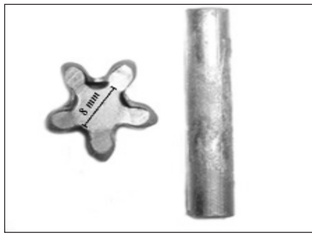
Fig 3. The billet and the precision forged gear.
