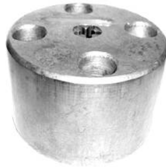
Fig.2. The die cavity used to forge spur gears. Fig.2. The die cavity used to forge spur gears.
