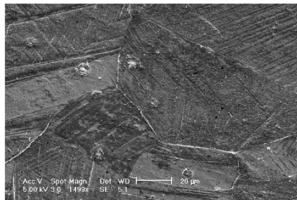
Fig. 6. Surface morphology of sample plasma nitrided at 420°C for 16 h.
