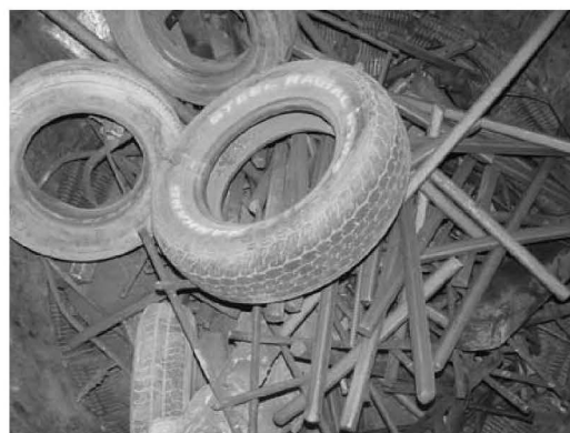
Fig. 4. Charging of scrap tires in the scrap basket.
