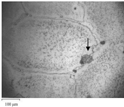
Fig. 6. Coarsening of carbides at grain boundaries after 120 cycles.
