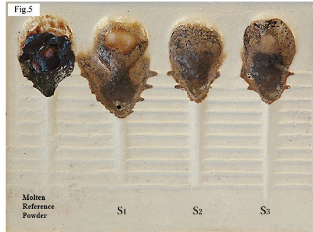
Fig.5. Schematic of molten samples of reference powder, S_1 , S_2 and S_3 on the grooves of the groove viscometer.
