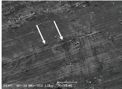
Fig. 10. Scanning electron microscopy image of from the worn surface of NiCoCrAl coating indicating the holes (shown by arrows) created by dislocations aggregation.
