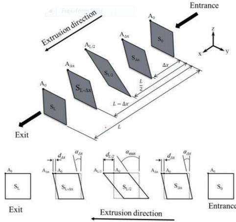
Fig. 1. Schematic illustration of the SSE process <sup>4)</sup>.
