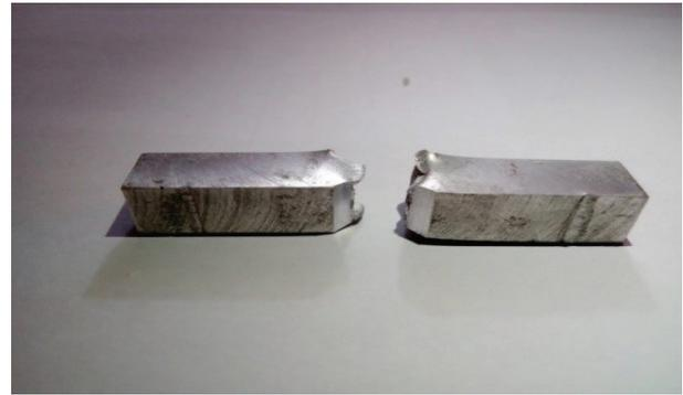
Fig. 8. Sample after impact test.
