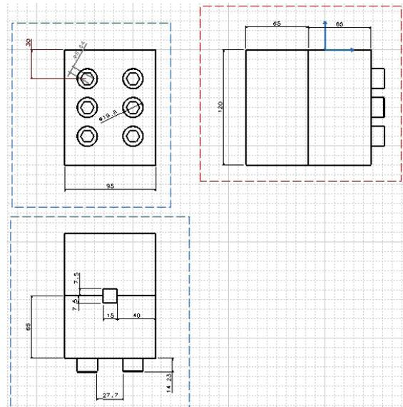
Fig. 2. SSE mold design by Catia software.
