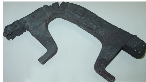
Fig. 4. Appearance of an amortized grate bar part.
