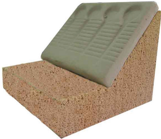
Fig. 1. Schematic illustration of the groove viscometer placed on the 45° slope.
